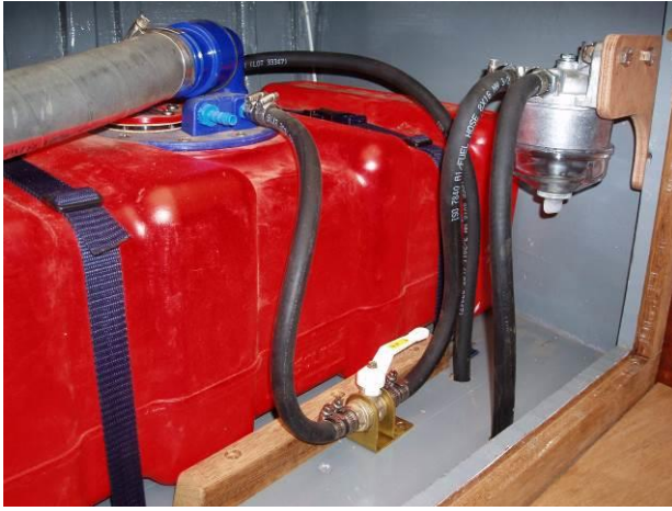
Pre-filter, shut-off valve and fuel pipes are fitted to the, now secured, fuel tank. The filter was later moved elsewhere to be lower than the tank.
