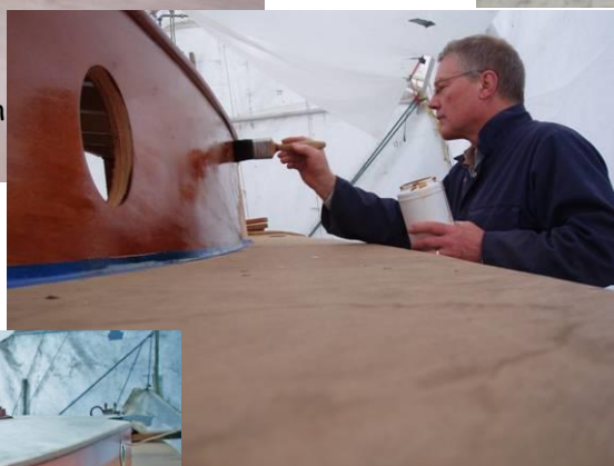
The cabin sides and cockpit coamings get their first coat of Sadolin Ultra Woodstain ...
