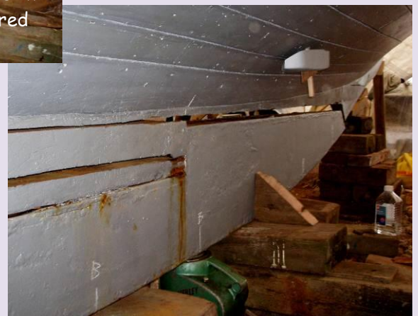
The cast iron keel is lowered using hydraulic jacks
