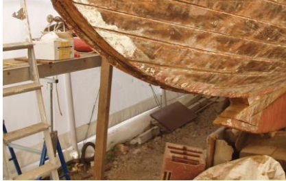
Old stem post removed, new post laminated and fitted with new bronze studs. Old breasthook 'exploded' by rusting stem bolt. New breasthook.
