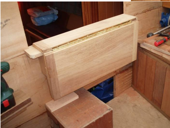
I didn't want washboards and so we start the development of a drop-down, folding, companionway door & step
