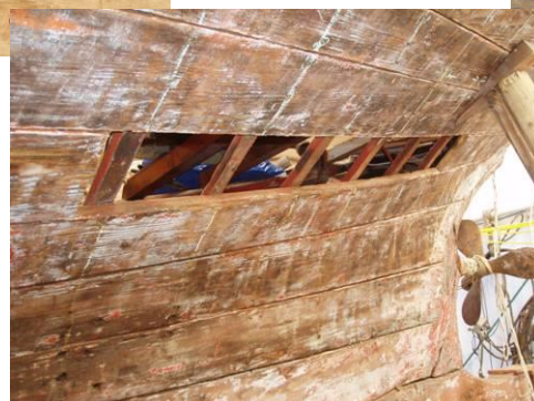
A damaged plank section removed and a new piece scarphed in. Temporarily screwed in place - copper nails and roves to follow..
