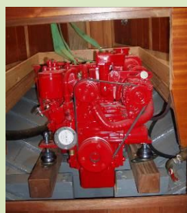
A Beta 20hp, 3 cylinder diesel unit, based on a Kubota block; indirect seawater cooled through a heat exchanger and freshwater tank. Lifted in on the long arm of the JCB and transferred to my electric hoist. Bolted down onto the engine beds and connected to the prop-shaft with a flexible coupling and clamped on shaft flange.
