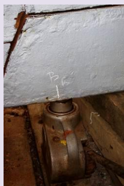
Sleepers & 'sledges' in place ready to receive the lowered 1½ ton cast iron keel.
