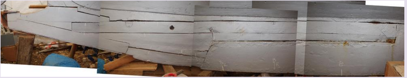
A composite showing the keel timbers that need to be replaced with new oak.
