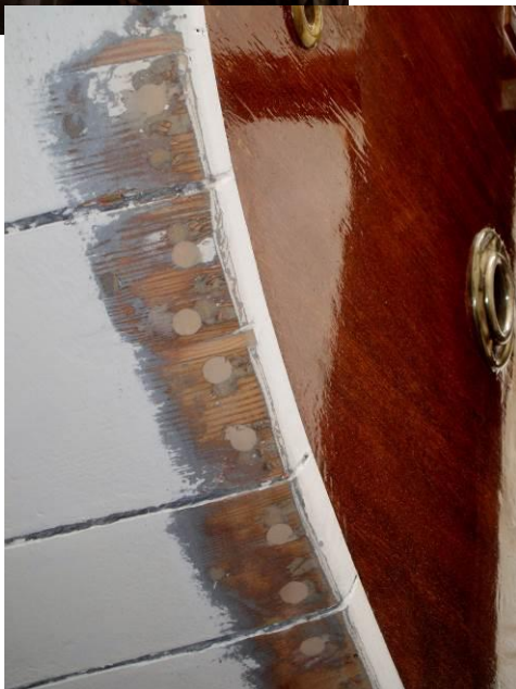
The surveyor recommended that the hood end and garboard fixings are doubled-up to ensure as little movement as possible. 170, 1 \frac{3}{4} " No.10, bronze screws are inserted!
