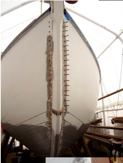
The surveyor recommended that the hood end and garboard fixings are doubled-up to ensure as little movement as possible. 170, 1 \frac{3}{4} " No.10, bronze screws are inserted!
