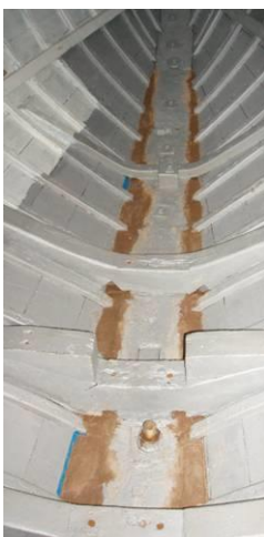
New cement infill, to replace the old concrete, between the hog and garboards along the full length of the boat
