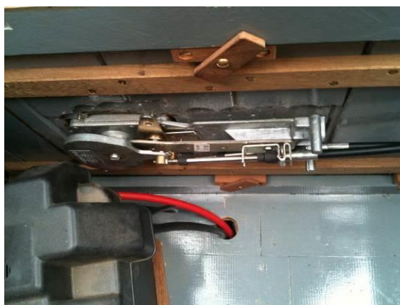
Engine gear & throttle control lever and cables are fitted
