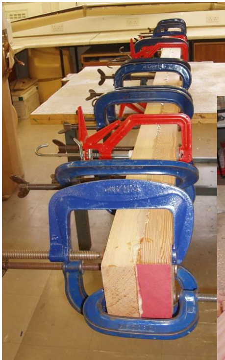
The 3m top section to repair the broken mast begins to take shape
