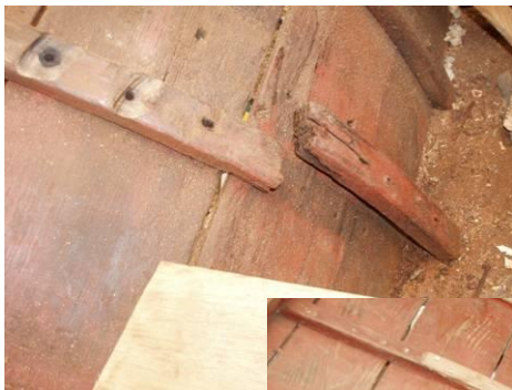
Broken frame sections removed and replaced with laminated Elm
