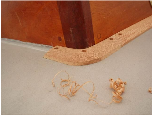
Making and fitting the moulding to seal between the cabin coamings and the deck
