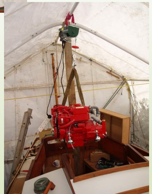
A Beta 20hp, 3 cylinder diesel unit, based on a Kubota block; indirect seawater cooled through a heat exchanger and freshwater tank. Lifted in on the long arm of the JCB and transferred to my electric hoist. Bolted down onto the engine beds and connected to the prop-shaft with a flexible coupling and clamped on shaft flange.
