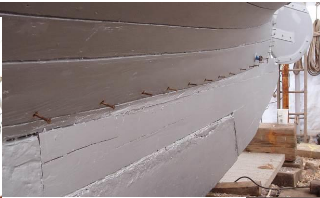
The surveyor recommended that the hood end and garboard fixings are doubled-up to ensure as little movement as possible. 170, 1 \frac{3}{4} " No.10, bronze screws are inserted!
