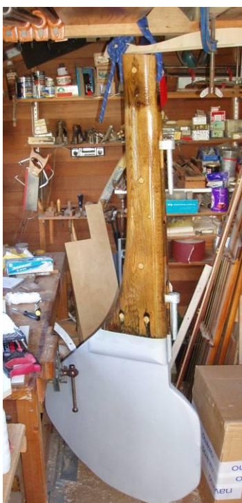
The restored rudder gets some paint and varnish before it & the new tiller are tried in place
