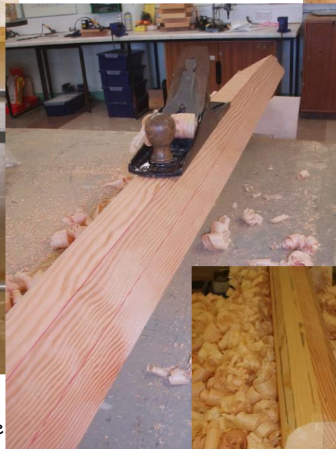
The 3m top section to repair the broken mast begins to take shape
