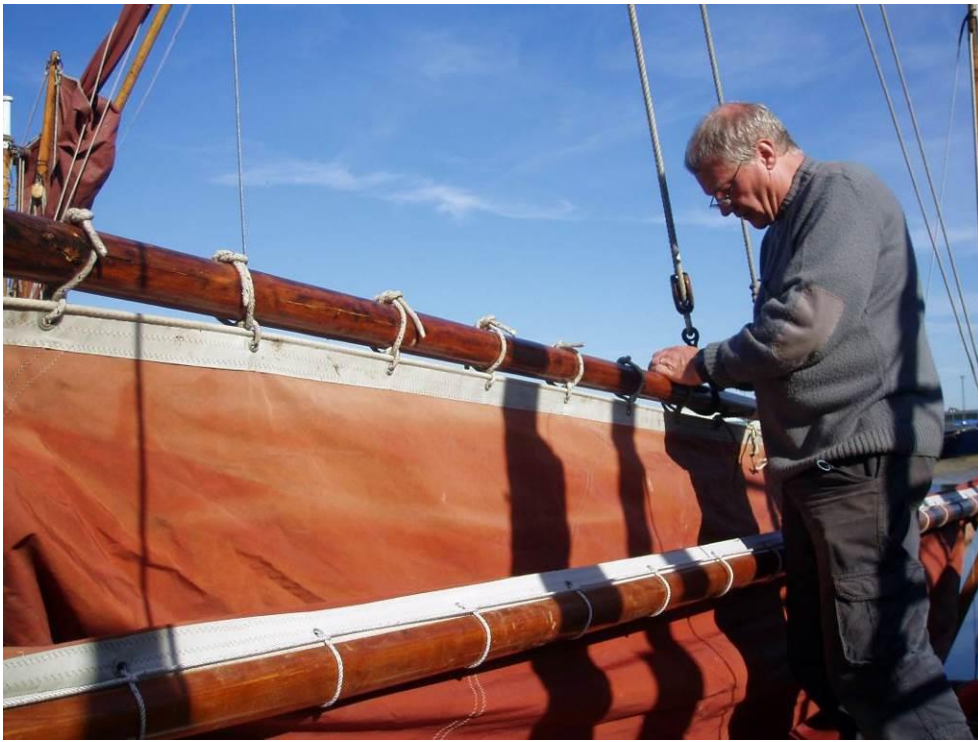
Sails are bent to the spars and the jib, with its Wickham-Martin furling gear, attached to the traveller on the Bowsprit.
