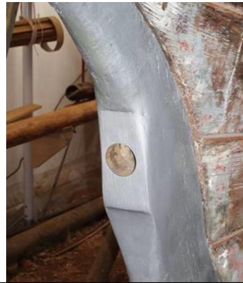
New piece cut in for the stern tube on the stern post
