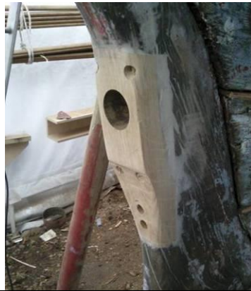
New piece cut in for the stern tube on the stern post
