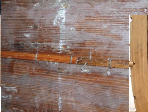
Broken frame sections removed and replaced with laminated Elm
