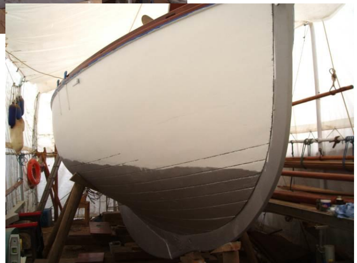
May 2013 - Barbara helps fill and rub down the remainder of the 2800ish nail holes and the primer coats are applied.
