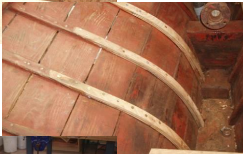
Broken frame sections removed and replaced with laminated Elm
